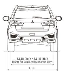
All measurements in millimeters
