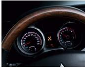
High-contrast back-lit meters and 22 gauges with tachometer, 4WD position display and rheostat
