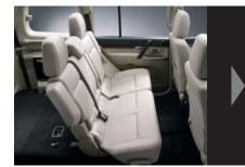
To provide as much carrying space as possible, the 2nd-row can have the seatbacks folded down, and then the seats themselves folded up and out of the way. You can also fold down just one part of the 60:40-split 2nd-row for carrying extra long cargo\*.
