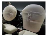
Driver's and front passenger's front SRS airbags (dual-stage)
