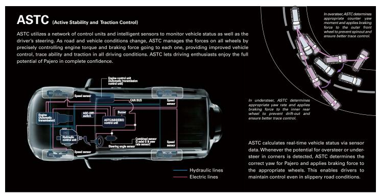
Note: The control capabilities of ASTC are supplemental only. Please drive safely and never rely solely on these functions while driving. Be sure to us the same specified type and size of tires on all 4 wheels. Do not install any aftermarket limited slip differential on your vehicle. Please see the owner's manual for additional information
